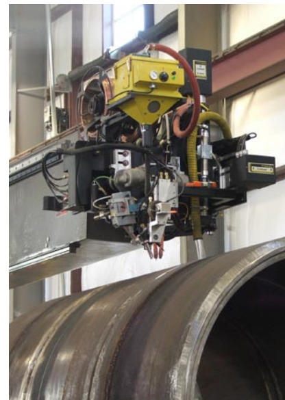
The design of AMET welding equipment is largely dictated by the techniques required to create massive wind turbine towers that can be nearly 90 meters high.
