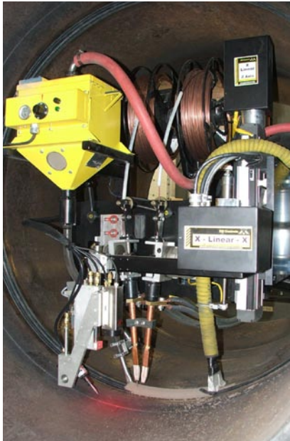
While the bulk of the welding equipment remains stationary during a weld, the weld head constantly moves small distances along at least 2 axes, both along and across the seam.
